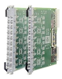
Left to Right; 20-Port 10BASE-F SwitchModule, 10-Port 10BASE-F SwitchModule.
