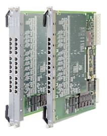
Left to Right; 24-Port 10BASE-T SwitchModule, 12-Port 10BASE-T SwitchModule.
