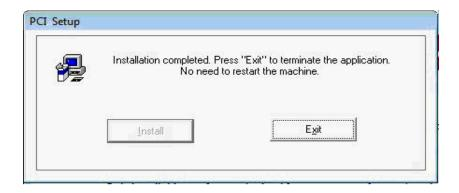
• Click on "Exit" and shutdown the PC. Place the MCS9865 based PCI card into PCI slot and then power on the system. After the system boots, the drivers are installed automatically and the status of installation can be viewed in the taskbar.
